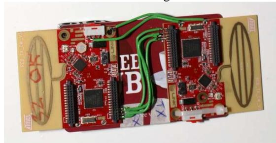
Fig. 2. The physical jamming hardware used has two radios present. One radio is always in the receive state, and the other always ready to transmit. This dual-radio configuration is faster at transmitting a colliding signal than using a single radio and switching between receive and transmit states.
